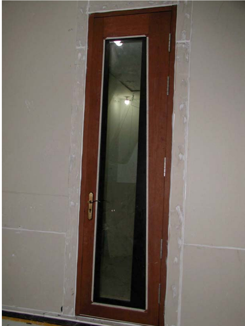
Figure 2 : Test set up of sample in the reverberation room
